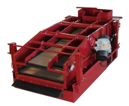
Scomi offers a comprehensive range of Solids control equipment for oilfield applications. The Scomi line of high-performance shakers are specifically designed and engineered to efficiently and reliably separate solids from drilling mud thus reducing waste volumes and associated costs.
